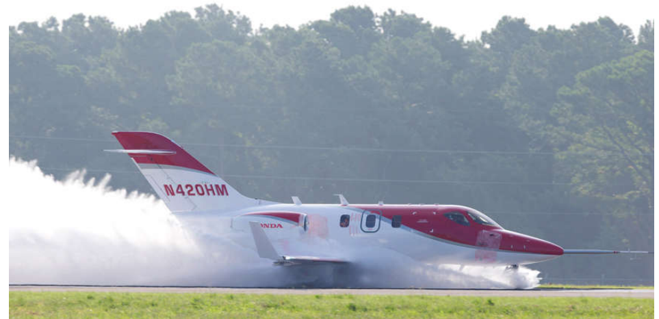
Wet runway water ingestion test of Honda jet. Photo: https://hondanews.com/hondajet/photos
